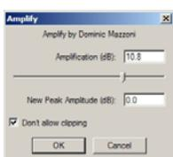
**Effect | Amplify** – accept the default suggestion in the dialog box. Ensure that "Don't allow clipping" is ticked – this will ensure that the overall range of the selection does not distort.
